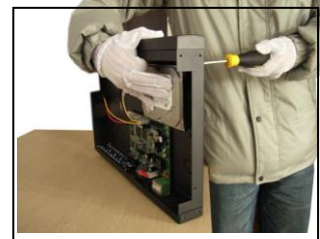
③fix the screw of the hard disk
