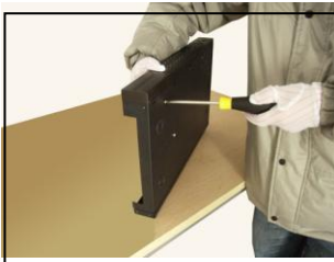
④fix the screw of the hard disk
