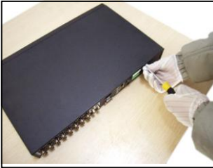
①disassemble the screw
