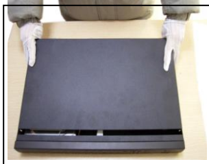
②disassemble the cover
