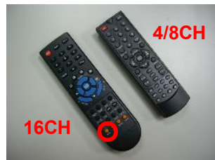
3. IR Remote Control * 16CH: Pressed "DVR1" Button before use
