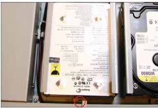
Place the mobile rack back onto the device and screw in the screw.
