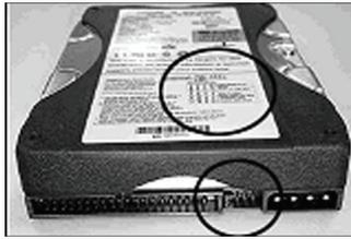
Setting the jumper of your **HD2** driver: The way to set the jumper of the drive varies between manufacturers; please refer to the instructions on the driver to set the jumpers in the **slave** position.
