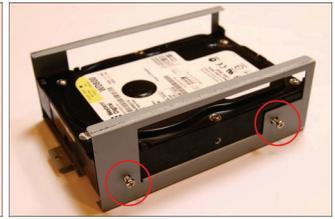
Secure the driver in the rack using 4 mounting screws in the side-mounting holes. Please don't tighten the screws too much, otherwise that may damage the driver.
