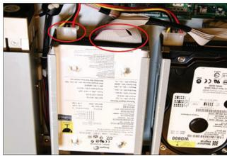
Attach the interface connector and the power connector to the drive. Please note the red lining of the IDE cable and the red wire of the power cable must line up side by side.
