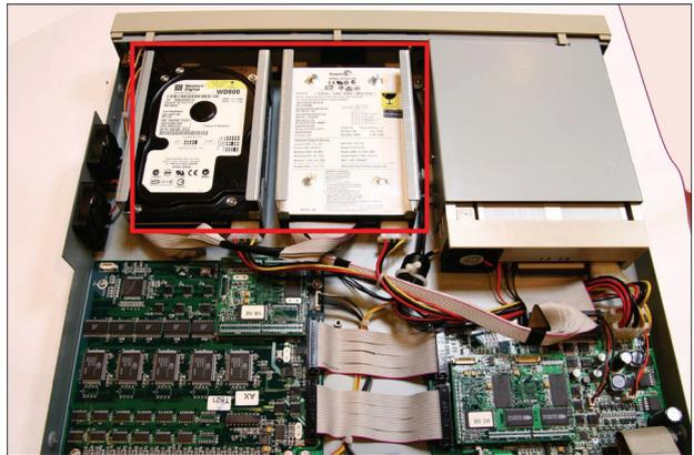
The installation of the hard-disk drive is complete.
