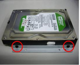
Step 2) Place the HDD on the HDD plate and screw it as indicated.
