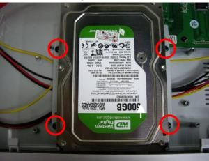
Step 3) Connect the power and the SATA cables as indicated.
