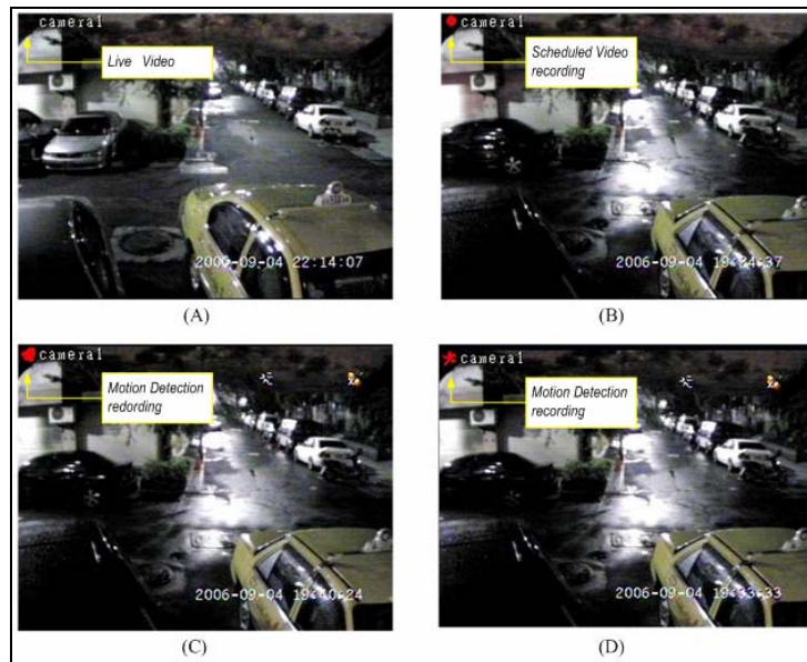
FIG 4 The icons involved in classifying the video: (A) the regular video; (B) Scheduled recording video; (C) Alarm detected video; (D) Motion detected video.
