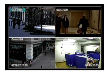
The split-window screen, as shown above, is the main screen after system startup. There are two types of split-window screens, including 1-Window and 4-Window. The system will remember the last one before normal shutdown (as described in <u>Section 5.6</u>) of the system. In addition to the split windows, the system time is displayed on the lower-left corner, the system states on the lower-right corner, and the rolling screen messages, if shown while certain event occurs, on the lower corner.
