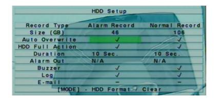
In the surveillance applications, alarm video/audio is much more important than normal video/audio. So, this digital video/audio recorder is designed to allow the user to divide each HDD into alarm partition and normal partition. And, alarm video/audio will be recorded in alarm partition, normal video/audio in normal partition.
