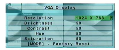
There are 5 items which can be adjusted, including Resolution (1280x1024, 1024x768, 800x600, 640x480), Brightness, Contrast, Hue, and Saturation. The operations are as below:
