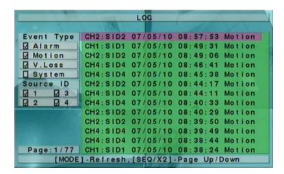
There are four different types of event logs, including Alarm, Motion, Video Loss, and System. And up to 1000 most recent event logs can be stored in the system.
