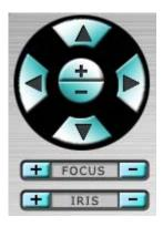
**PTZ** control panel. If the camera in the focus window is a PTZ camera, these buttons in the PTZ control panel can be used for PTZ control. The operations include Tilt Up/Down, Pan Left/Right, Zoom In/Out, Focus Near, Focus Far, Iris – (darker), Iris + (brighter).
