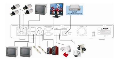
Please make sure to set the NTSC/PAL Selector Switch on the back panel according to the local TV system for the system to work correctly.
