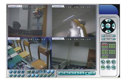
The video images can be displayed in several types of split-window screens, including 1/4/9/16-Window. And the focus window is surrounded by a frame border. In addition to the video windows, there are different icons on the lower corner and the right corner of the screen for status display and control. (The ".L" following the camera title stands for Live display, ".P" for Playback, and the camera title with white background has detected motion.)
