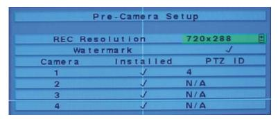
There are up to 4 cameras which can be connected to the system. The Pre-Camera Setup allows the administrator to define some fundamental attributes for all the installed cameras.
