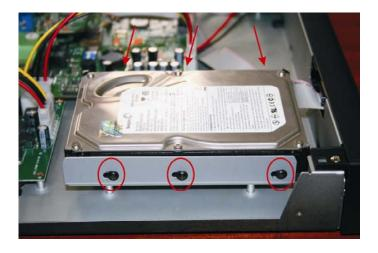
3. Connect the cables (3.5 " HDD) as shown.
