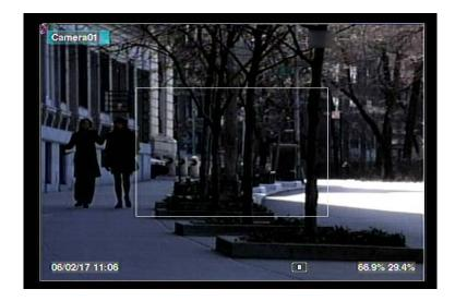
The system supports X2/X4 Digital Zoom function. To use this function, press **X2** button in full screen display to enter Digital Zoom mode. There will be a zoom window shown in the video window as shown. The zoom window (a) will always be shown at zoom factor X1, (b) can be shown or hidden at zoom factor X2, and (c) will never be shown at zoom factor X4. The operations in Digital Zoom mode are as below:
