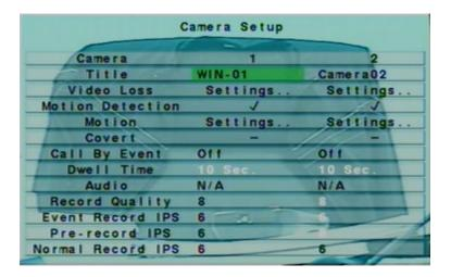
The Camera Setup allows the administrator to define the attributes for each camera. There are up to 4 cameras which can be connected to the system.
