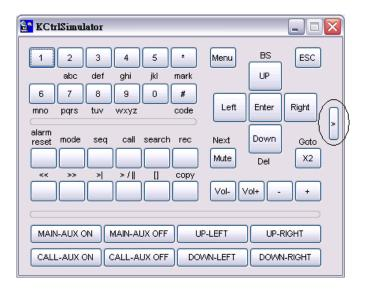
Please note that most of the buttons correspond to the keypads on the front panel. If you connect the PC through RS-232 and use an RS-232/RS-485 converter to connect to multiple DVRs, you would be able to control multiple DVRs via the simulation software. Please refer to Section 3.2 Optional Connections to connect/cascade the DVRs to the PC.
