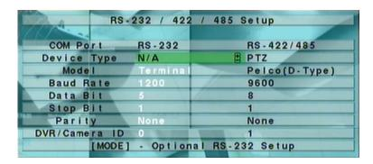
The RS-232/422/485 Setup allows the administrator to setup RS-232 control port, and RS422 or RS-485 control port. Please refer to the manuals for the connected devices - PTZ cameras – to set these items in RS-232/422/485 Setup.
