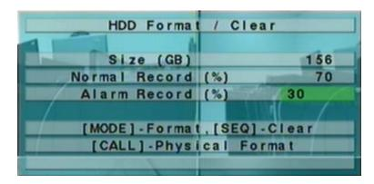
The HDD must be formatted before it can be used to record video/audio. The HDD Format/Clear screen allows the administrator to format and/or clear each HDD, and set the size for Alarm Record partition and Normal Record partition for each HDD. Please use only HDD with maximum storage size as 500GB, and make sure there's no remote user before formatting the HDD.
