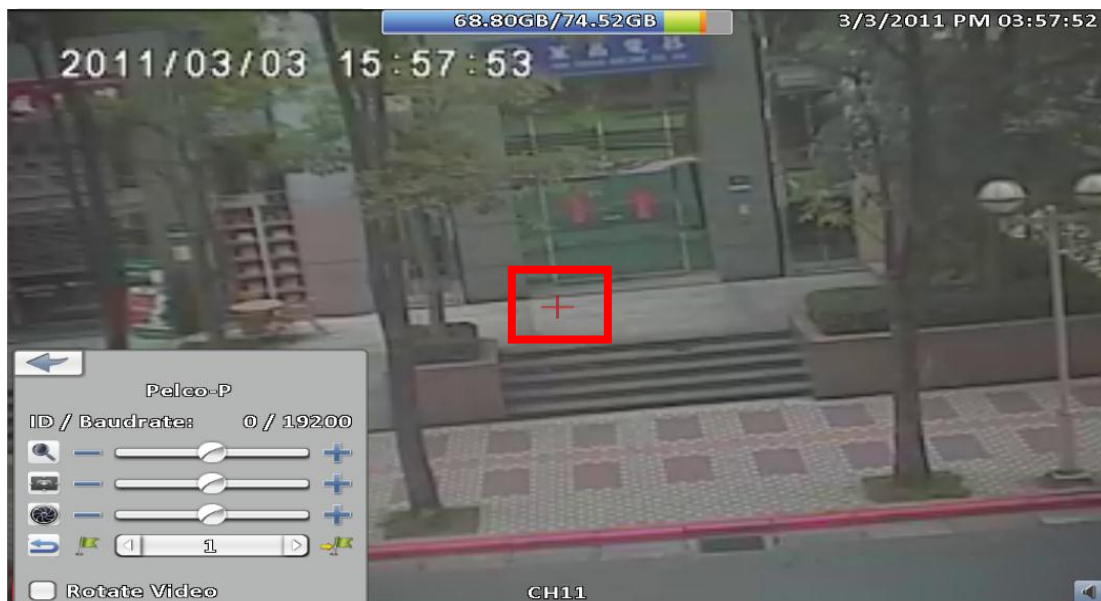
4:3 display mode of operation of PTZ functions
