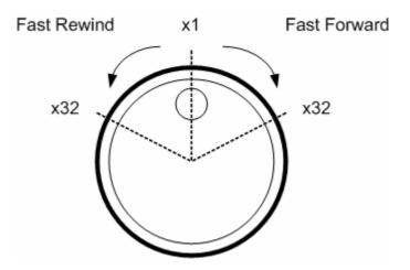
Inside the shuttle ring is the jog disk, shown as the figure, it can turns completely in either directions. Once you freeze the video, you can use the jog disk to go single-step playing back. Clockwise rotation causes a forward one-step playback; and counterclockwise rotation causes a backward one-step playback.
