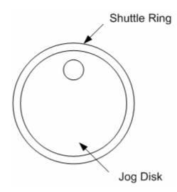
While playing back video, you can use the shuttle ring to select different speed of forward and backward playing. Rotating the shuttle ring counterclockwise causes the unit to playback into faster forward/ backward playing speed. According to the angle you rotate the shuttle ring, you can choose the playing speed from 1x, 2x, 4x, 8x, 16x, and 32x, in both forward and reverse directions, shown as below figure:
