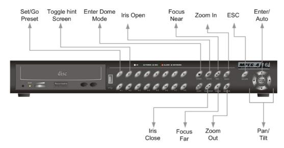
The function keys used in Dome Control are described as follows.
