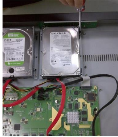
Step 5. Connect the SATA cables to the SATA connectors on the main board. Please refer to the below for the hard drive port numbers and connect the HDD accordingly. The DVR will recognize the hard drives according to the SATA port numbers for the disk management.
