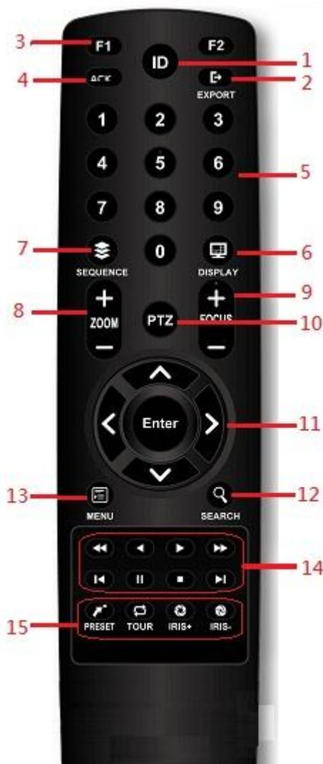
1. **ID Button:** Press ID button + number key to switch to the DVR that user would like to control. Press a number between 1 and 9 corresponding to the unit ID you wish to control. The user ID must be set in the device before operating.
