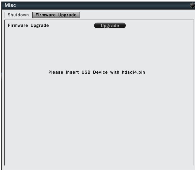
To upgrade the firmware, connect a USB flash device which contains the firmware version you would like to update. Click “Upgrade” to start the firmware upgrading. The system reboot is required to complete the firmware upgrade.
