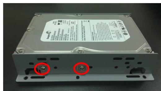
Step4. Connect SATA & Power wire to Hard Disk and put it on right position of the case. Use the HDD mounting screws attached in the accessory pack to fix the hard drive with bracket firmly on to the chassis.
