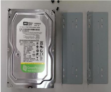
Step 2. Fix the harddisk on to the harddisk mounting bracket and fix the screws on to the screw holes as indicated in the diagram. Each set of harddisk brackets can mount 2 harddisks.
