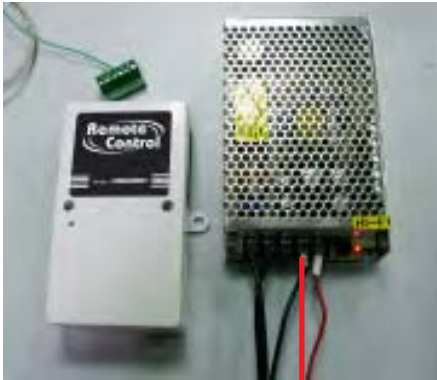
Connect to DC power supply (Power consumption: 12VDC)
