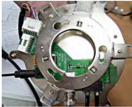
Picture 3: Connectors at the front side of PTZ camera base
