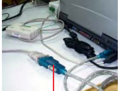
Connect to USB/RS232 converter (DVR without COM Port)
