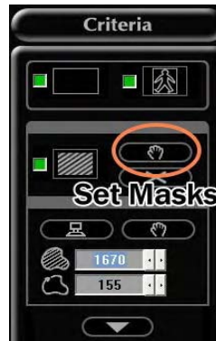
Set non-segmentation area. Up to 10 mask areas can be used. Use mask for unstable background (ex: leaves, flags) to avoid incorrect calculation. Mask area will display as negative image frame.
