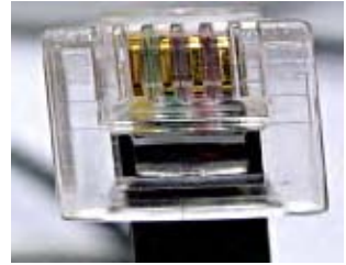
Picture 1: RJ11 connector (four lines inside)
