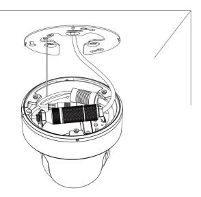
Step2: Rotate the camera to bracket and tighten the setscrew;
