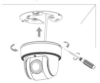
Step3: Loosen clamp screw and adjust shooting direction, tighten clamp screw.
